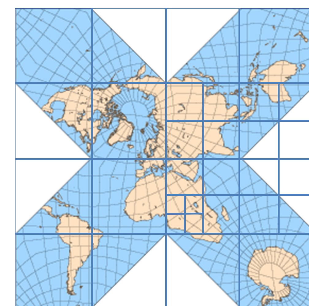
An illustration of "Butterfly HEALPix" projection, and the hierarchical spatial partitioning of database tables into cells
